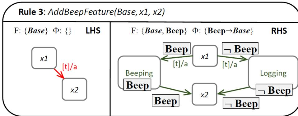
Figure 3.2: Transformation rule for adding the feature *Beep* to a software product line
